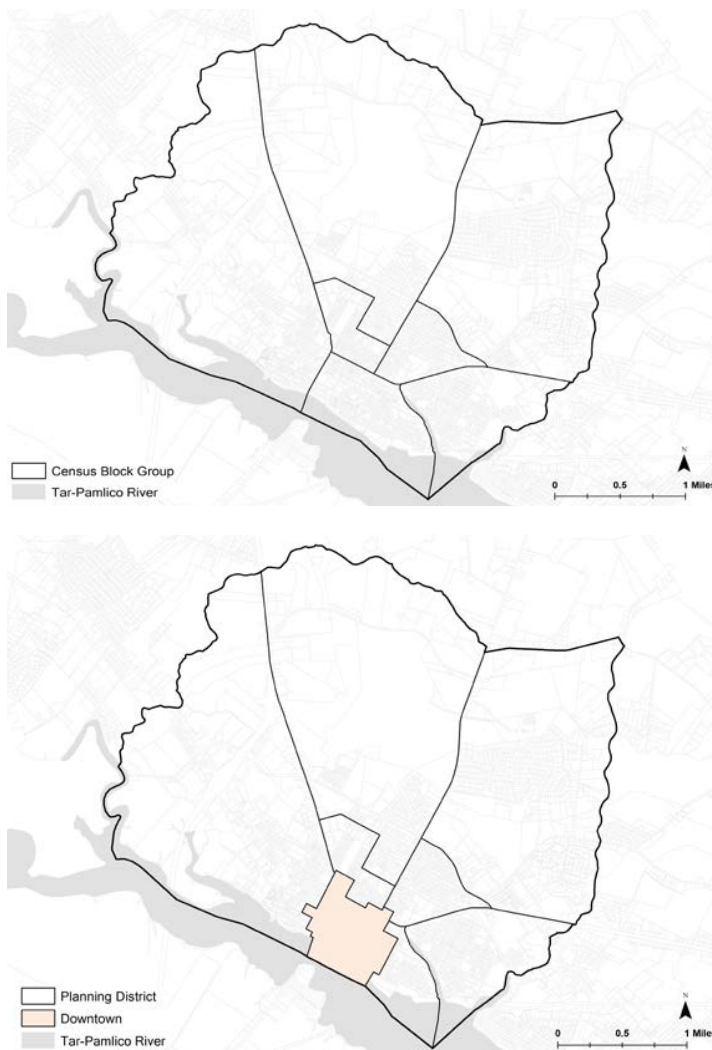
Figure 2.3 Customizing Planning Districts. The map (right) displays Census block groups for Washington, NC. Because there was a strong focus on the central business district (CBD) in the plans, we created a customized planning district map. Using GIS software, the CBD is clipped out of the Census block groups to create a new geography.
